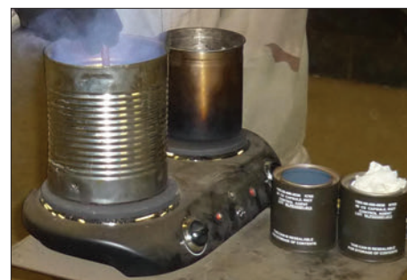
Hot plate method of CS dispersion at the Fort Jackson mask confidence chamber.
