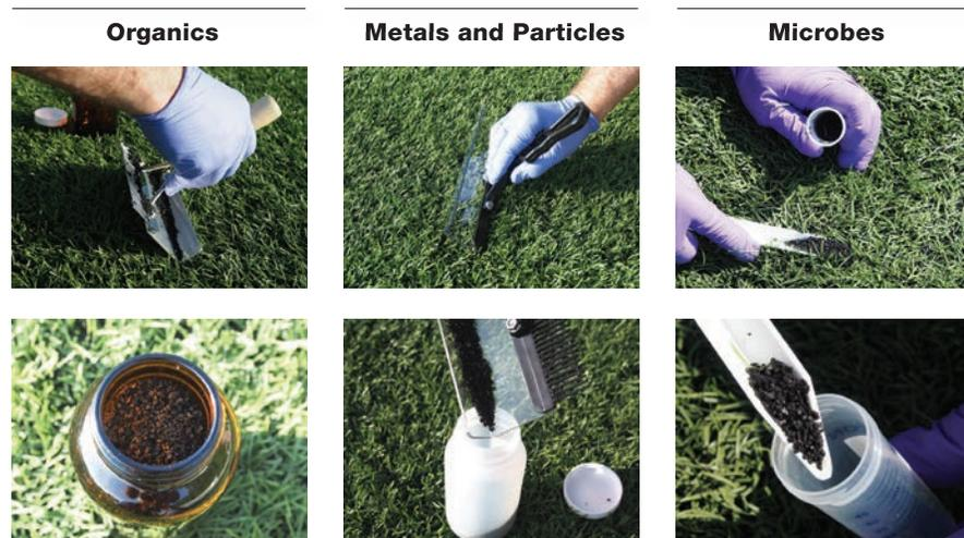
*Note.* Combs were used to sample for organics and metals and particles. Spatulas were used to sample for microbes. Samples were taken from approximately the top 3 cm of the synthetic turf field surface.
